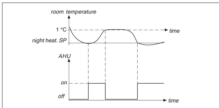
When the temperature has reached 1 °C above the night heating setpoint, the AHU stops. There is a choice of running only TF during night heating.
