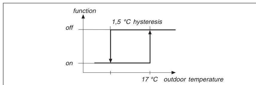
The circulation pump is restarted when the temperature is 1,5 °C below the “Outdoor temperature limit”, which is equal to the hysteresis.
