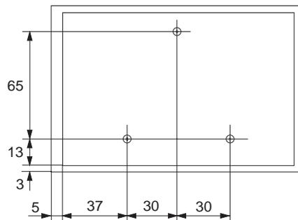
► **Procedure for mounting controller on a wall:**
