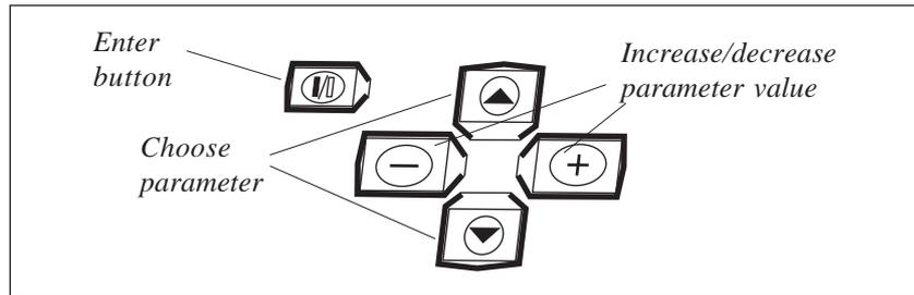
*The buttons on the operator's panel*
