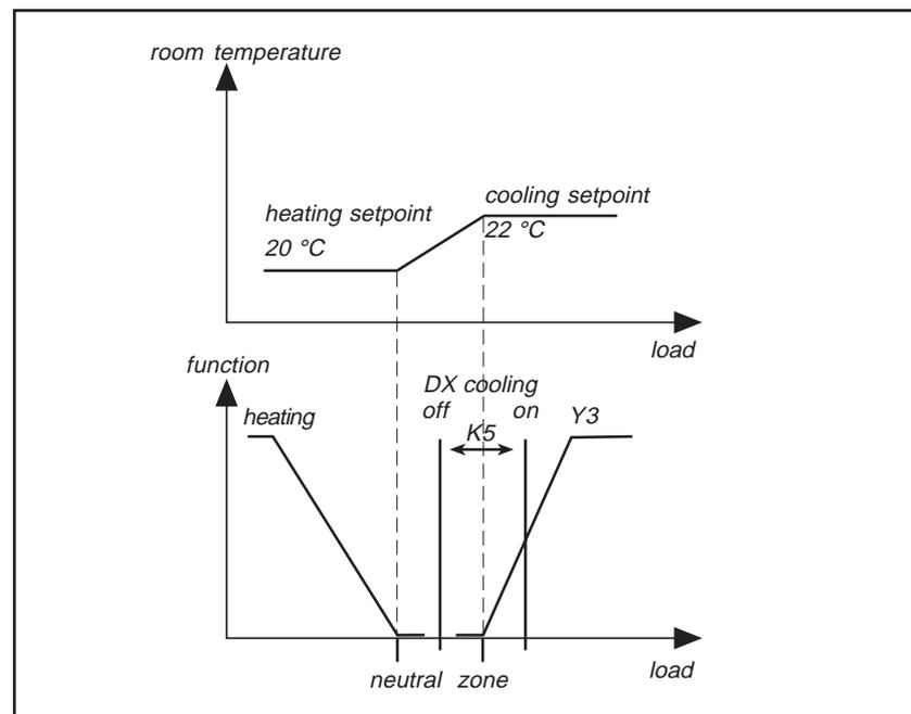
Example: If the cooling setpoint is 22 °C, and the heating setpoint is 20 °C, then the P band is 2.
