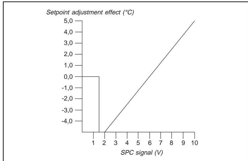
There is no change to the setpoint at 6 V, but 2 V and 10 V provides the set effect with a – or + sign. This means that 2 V will give the (–) effect and 10 V will give the (+) effect. However, an input signal that is < 1.5 V will achieve the same effect as 6 V, that is no change to the setpoint.
