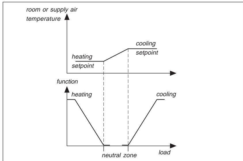
If the temperature lies within the neutral zone, neither the heating nor the cooling coil is active, see the figure above.
