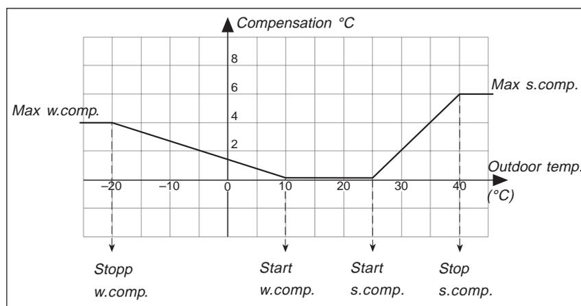
The outdoor compensation is not active on delivery. It is activated by setting the desired compensation values in the list, P 50 for winter compensation and P 53 for summer compensation.
