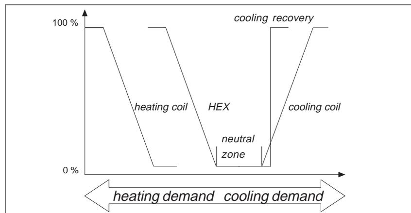
When there is a heating demand, the HEX increases the control signal to 100 %; then, the heating valve opens. During a cooling demand, the heating valve closes first, and then the control signal to HEX is decreased to 0 %. Only at this point does the cooling valve open.
